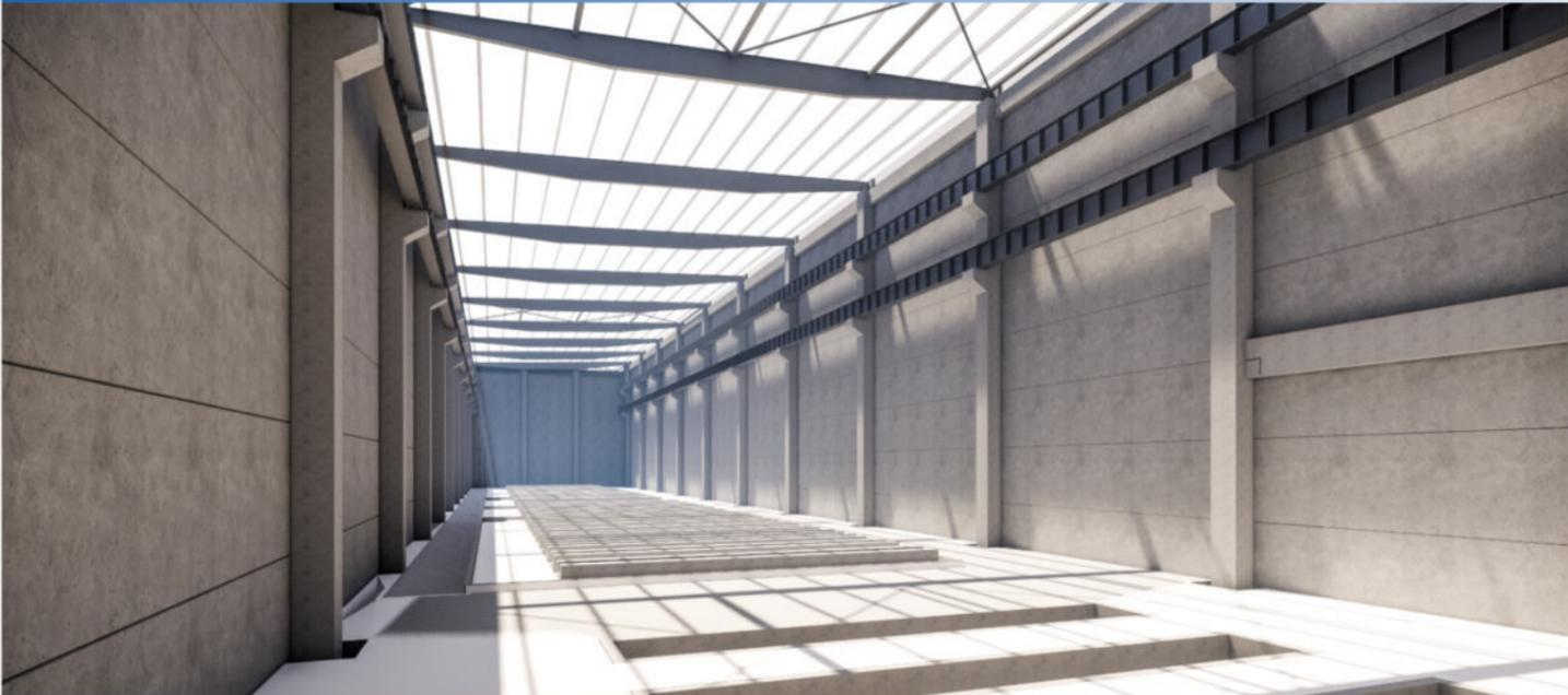
3D MODEL: DESIGN OF PRECASTE CONCRETE COLUMNS, WALL PANELS
